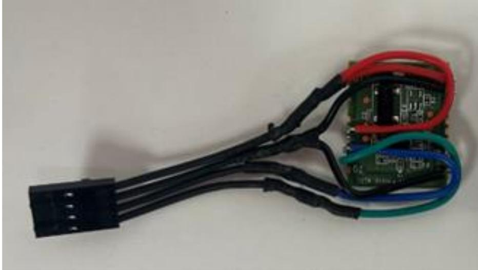
*Figure 7: IMU used for STEMnaut data collection.*
