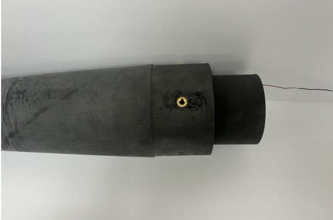
*Figure 21: Payload integration into rocket nosecone.*
