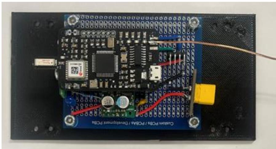
*Figure 4: 3D printed data transmission tray with electronics mounted on top.*
